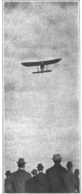
One type of Blériot monoplane, head on. Other type has spreading tail. Gnome motor. Planes slightly curved near front edge. Slight warp. Rear control. Always ready. Medium stability in the wind. Medium weight. When built for carrying capacity has larger planes more curved
